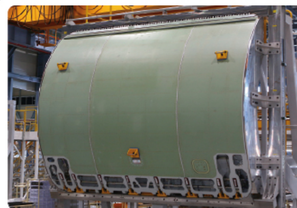
Main Deck Cargo Door
